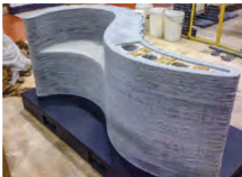
Fig. 3. A full-scale bench was created using concrete printing, incorporating post-tensioned reinforcement and functional voids
