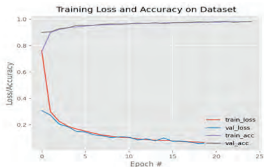
Fig. 5: Train and validation accuracy obtained through CNN Model
