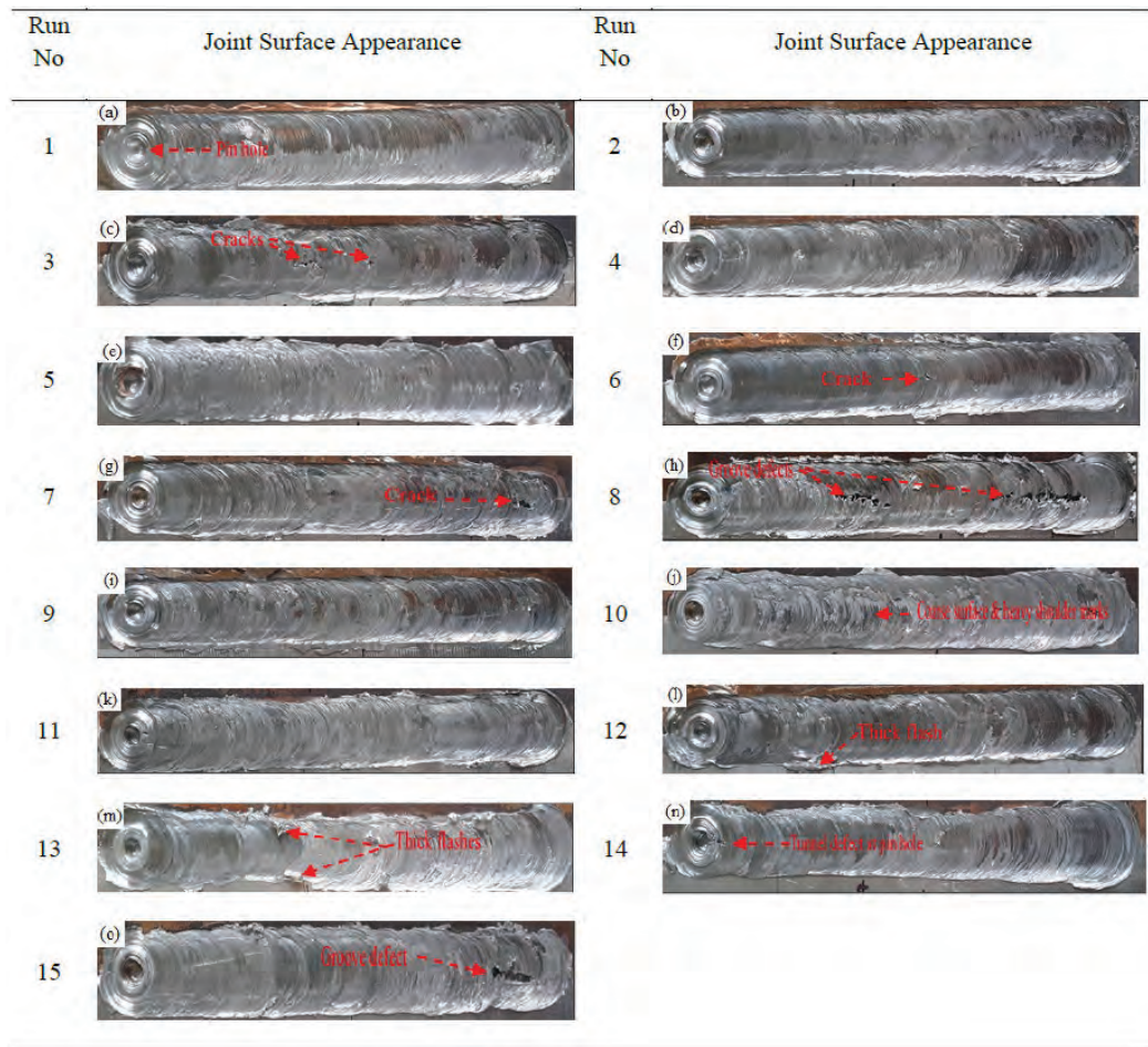
Fig. 3 Joint surface appearance and defects formed during the process
