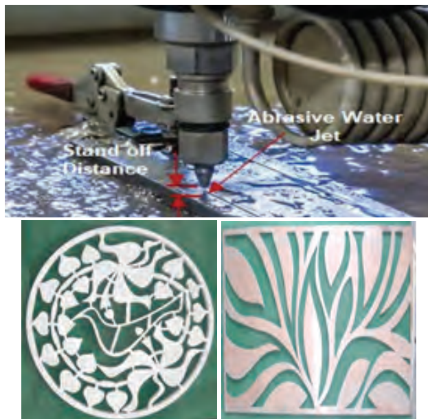
Fig. 1: AWJM Set up and Parts
